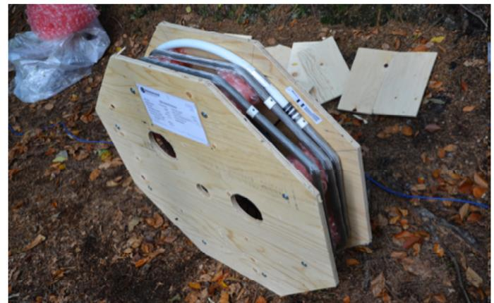
Fig.3 - 6 meters long SAA sensor (20 segments)
