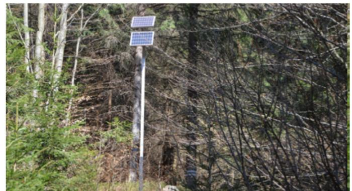
Fig.4 - Solar panels that supply the datalogger through battery
