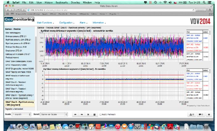
Fig.10 - "Historical Data" Rate of Change (RoC) in 24 hours interval at each segment. Horizontal lines are set alarms. Top Graph has an automatic scale, bottom one has the fix scale.
